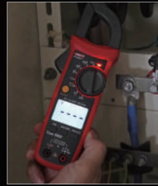
NCV multi-segment display and audio/visual alarm
